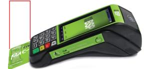
When a card is inserted, it slides further into the device than it normally should. The card should only slide in to read the chip.
